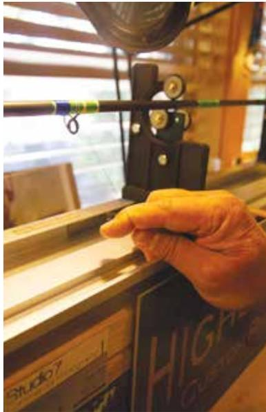
Rod, depending on the length, Amerongen uses between 12 and 16 guides including the tip top. Building a rod with more guides came after years of
